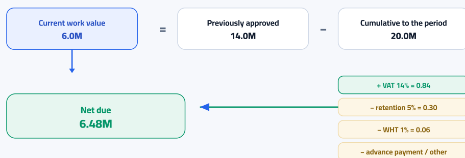
Figure 4 — Calculating the payment certificate: the cumulative minus the previously approved = the current, then adding VAT and deducting the retention, taxes, and advance = the net due
